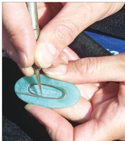
Score the cutting point with an X-Acto knife blade, then remove the wire to cut and solder it.
